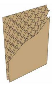
DIAMOND-PAK® bulkhead void fillers are used to fill a range of voids for boxcar, intermodal, ocean, and OTR needs. Lightweight and reliable, they provide an additional layer of load securement when used in conjunction with an air bag. These customized honeycomb panels provide significant strength and durability to withstand end-to-end impacts in boxcars.
